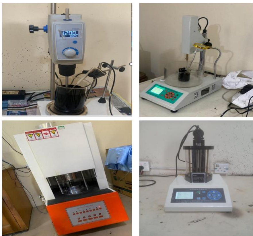
Figure 1. Laboratory equipment used for bitumen modification: (a) Variable speed high shear mixer (b). Asphalt Penetration tester (c). LR-A018 No Rotor Rheometer (d). Softening point analyzer (Bitumen Laboratory, Chemical Engineering Department, LAUTECH, Ogbomoso, Nigeria)
