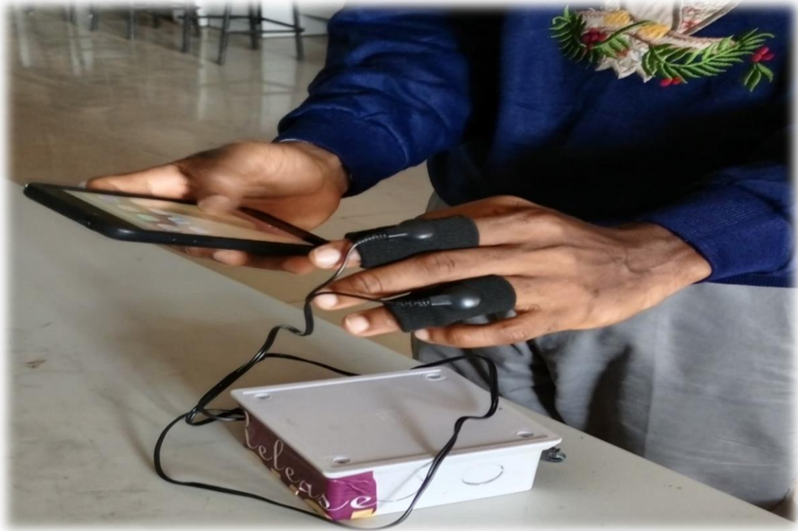
Figure 2. Measurements of body fat with two-choice finger and a Smartphone Interface
