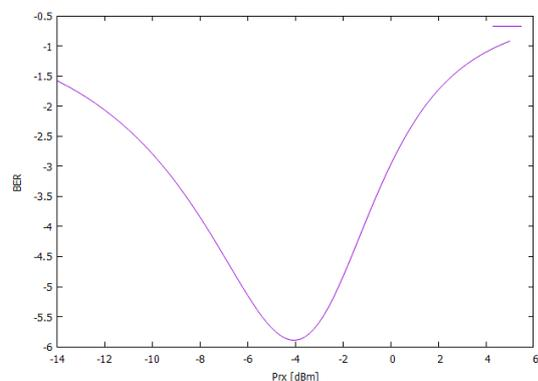
**Fig. 2. GN Model performance using Bit Error Rate**
