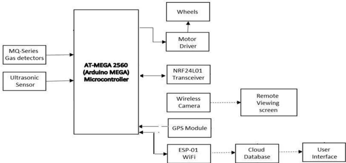
Figure 3: Block Diagram of Gas Detection mobile robot (Hardware)
