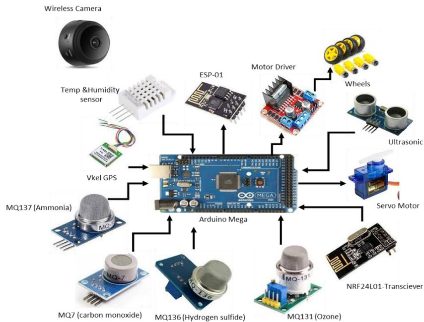
Figure 4: Component Composition of Gas Detection Mobile Robot (Hardware)
