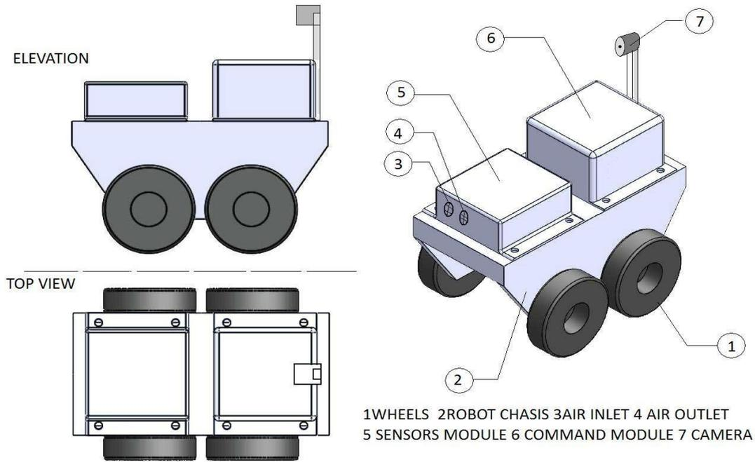
Figure 2: An overview of the Gas Detection Mobile Robot
