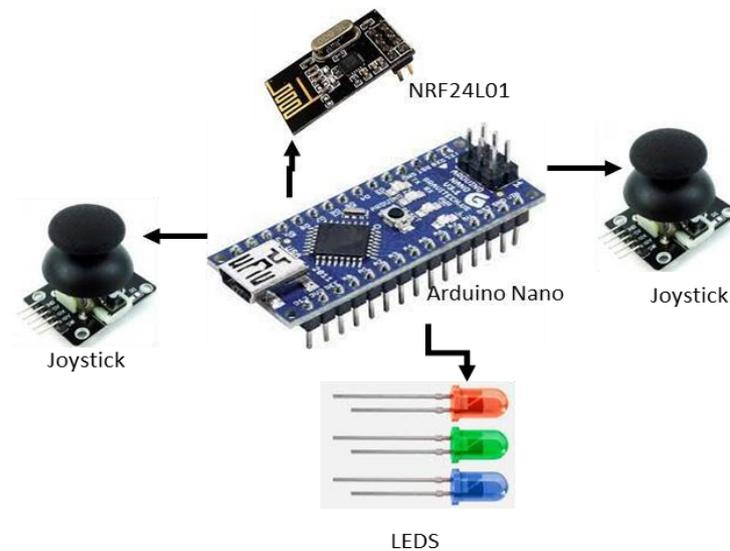
Figure 6: Component Composition of Wireless Remote Controller
