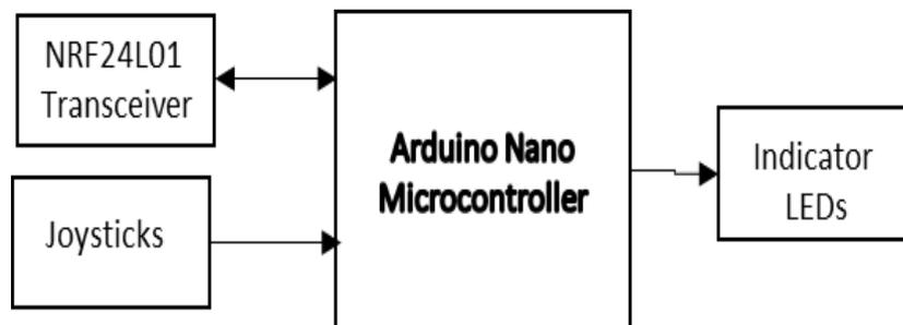
Figure 5: Block Diagram of Wireless Remote Controller
