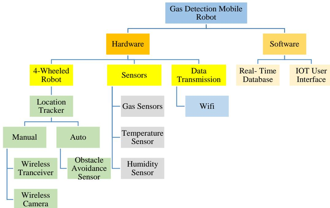
Figure 1: Overview of IOT-Based Gas Detection Mobile Robot
