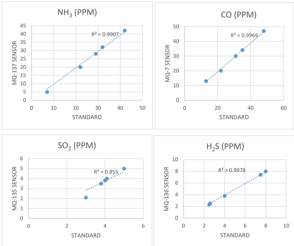
Figure 9: Correlation between gas concentration as measured by the standard gas detector and as measured by MQ Series sensors.
