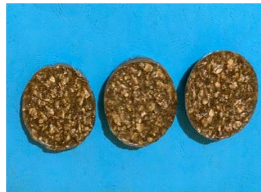
Figure 3: Corncob hybrid composite
