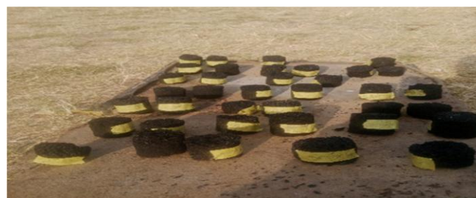
Figure 2: Charred cashew nut shell-sawdust composite briquettes
