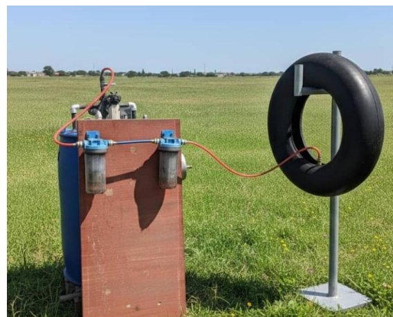
Fig. 6: The Fabricated Anaerobic Digester
