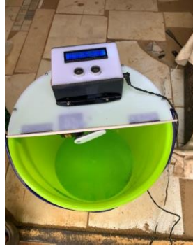
Figure 6: The opening of the smart dust bin for testing.
