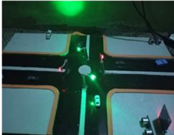
Figure 4: Density based traffic control system
