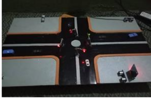
Figure 3: Arrangement of the Ultrasonic Sensors and RFID reader on layout
